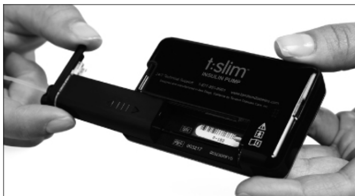
Cartridge being Inserted into t:slim Pump
