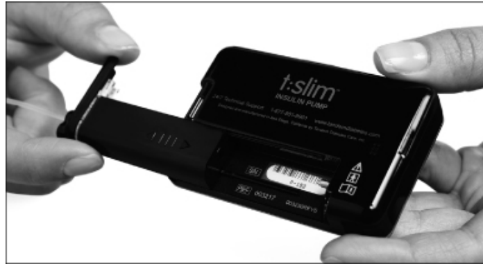
Cartridge being Inserted into t:slim Pump
